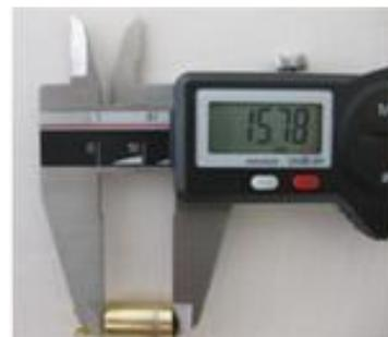
Atomizer, dimension of cutaway: 5,8 +/- 0,3 mm
