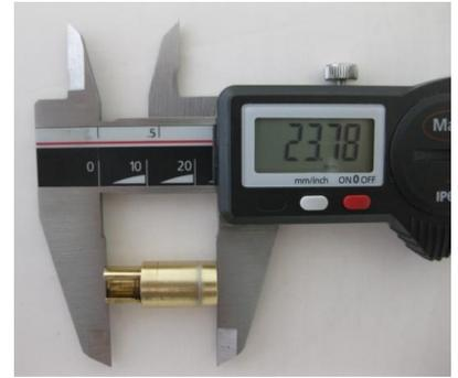
Atomizer, length of cylindrical part: 15,75 +/- 0,25 mm
