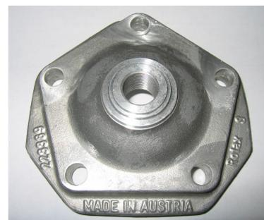
Height of combustion chamber insert has to be 28,80 mm +/- 0,2 mm (H).
