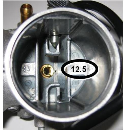
Angular bore of carburetor insert
