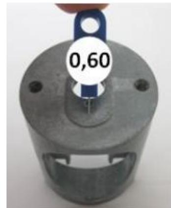
Vertical bore of carburetor insert
