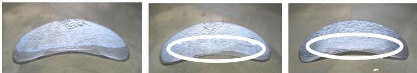
The exhaust port may show partial manual grinding done by the manufacturer to eliminate minor casting defects and/or to eliminate the NIKASIL burr at the end of the NIKASIL plating (right picture).
