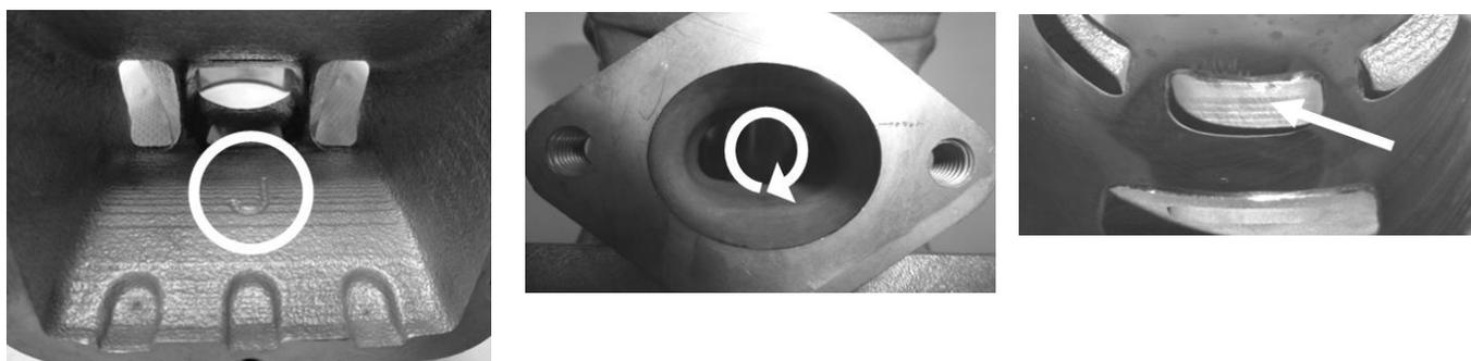
The horizontal and vertical dimensions of the exhaust port (cylinder 223 994 with fully CNC machined exhaust port only) have to be checked with the template (Rotax part no. 676 240). The template has to be moved in horizontal- and vertical position as far as possible into the exhaust port. In both directions the template may not touch the exhaust socket flange.
