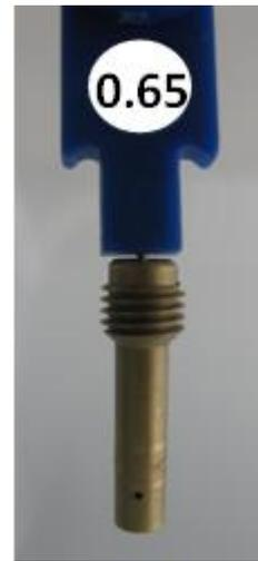
Plug gauge 0,65 mm may not enter one of the 4 cross bores (use jet gauge set Rotax part no. 281 920).
