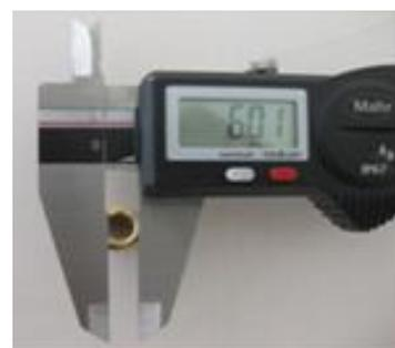
Atomizer, dimension of cross bore: 5,0 +/- 0,15 mm
