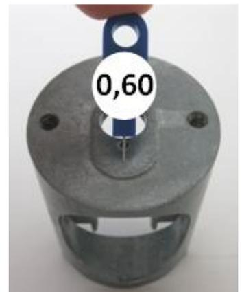
Vertical bore of carburetor insert
