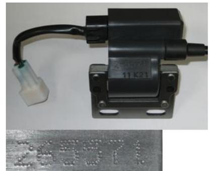
The ignition coil has to be fixed by means of 2 original silent blocks to the gearbox cover.
