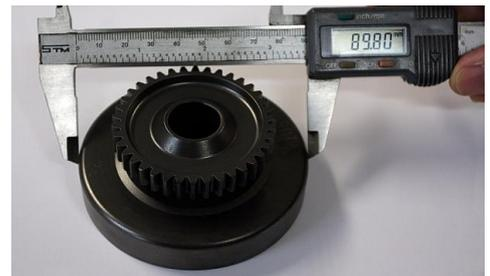
Inner diameter of clutch drum
