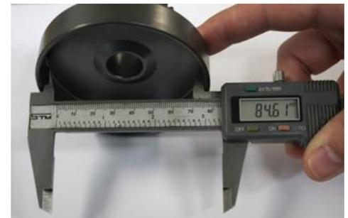
Height of clutch drum with sprocket/primary gear
