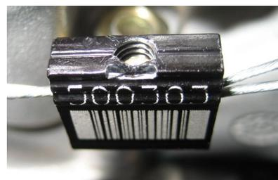
By means of the steel cable the engine must be sealed on one Allen screw (pos. 1) of the intake flange, on one stud screw (pos. 2) of cylinder and one Allen screw (pos. 3) of the cylinder head cover (see attached pictures).
