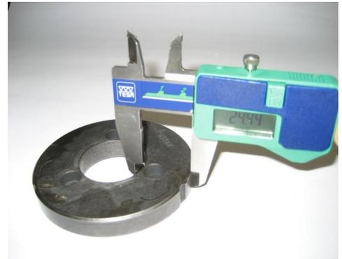
Outer diameter of clutch drum
