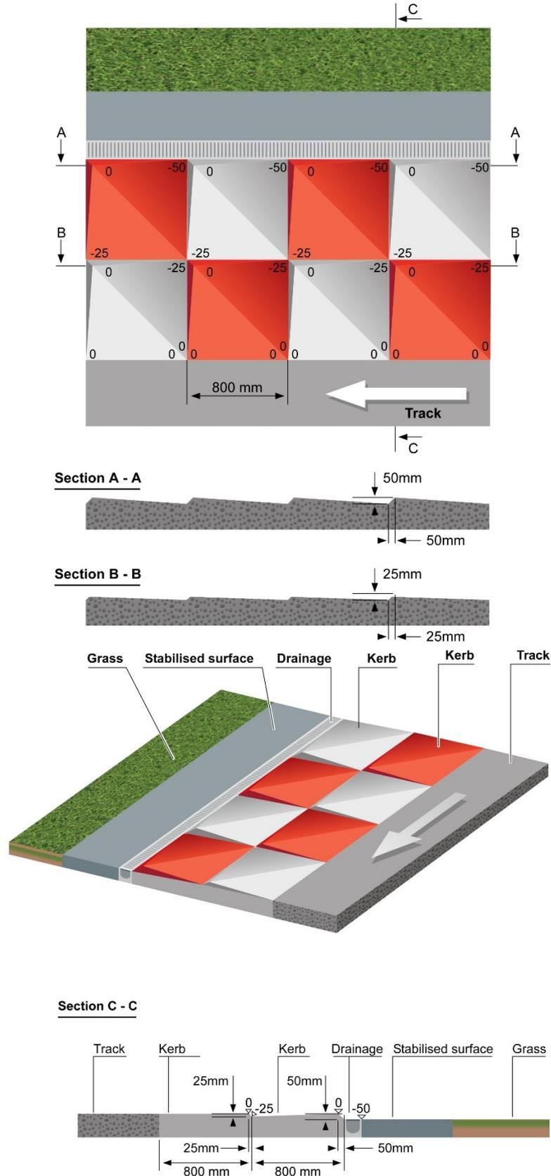
**Figure 6 Type 5 Double negative Kerb**
